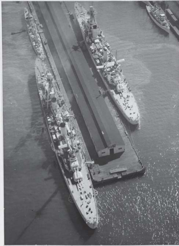
Figure 2. The French heavy cruisers Suffren (r) and Duquesne during a visit to Norfolk in October 1931. Note their four twin 8-in. gun turrets and the scouting floatplanes mounted on catapults abaft their funnels. Courtesy of www.history.navy.mil .
