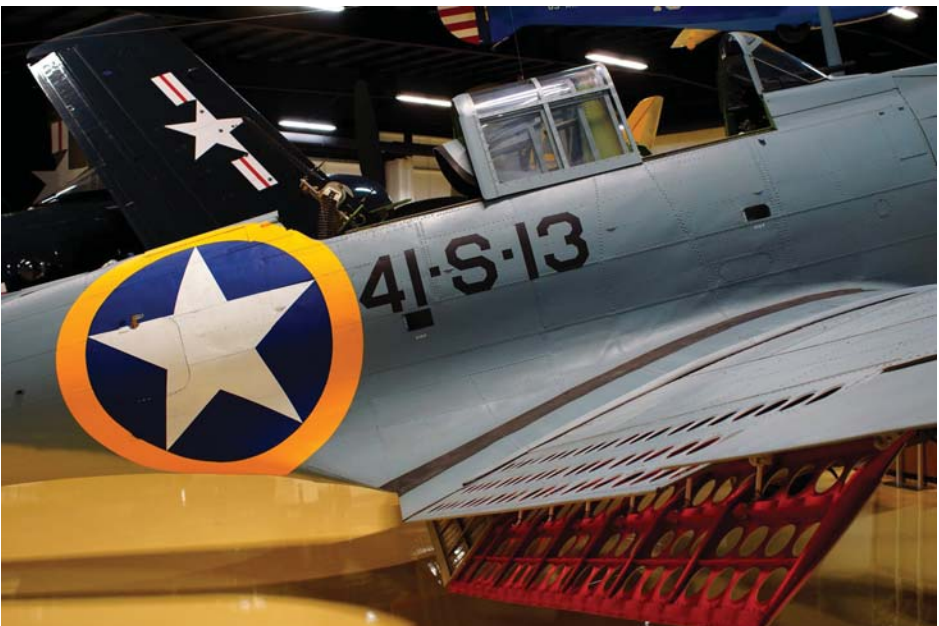
Figure 4. SBD-3 Dauntless BuNo. 00624. Note the perforated braking flaps. These slowed the plane's dive and provided the pilot with increased maneuverability. Photo taken by the author.
