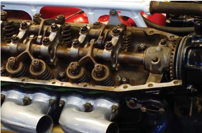
Figure 2. This image shows a section of the Allison V-1710 valve train. The Allison used a single overhead cam with four valves per cylinder. Ford Motor Company was the prime supplier of the R-2800 and they produced the engine in Dearborn, Michigan. Additionally, Continental Motors Corporation built the Merlin under license from Rolls Royce in Muskegon, Michigan.
